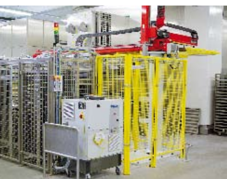
The robot for the automatic removal of unproofed dough pieces onto baking trays.
