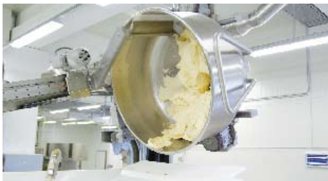
By means of a lift tipper with scraping device the dough is transported into the dough divider.
