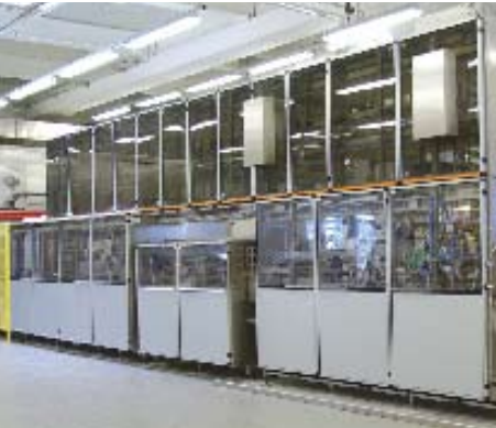
The multifunctional bread rolls line of W&P Kemper can stamp, press and round mould dough pieces.
