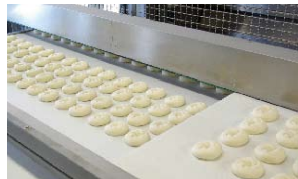
Completely proofed, the big volume dough pieces leave the proofer and are deposited onto the infeed belt of the oven loader by means of a crosswise retracting belt.
