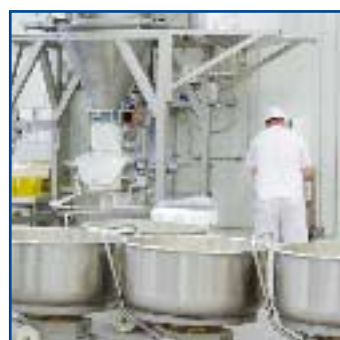
The dough preparation of the SPAR bakery in Ljubljana. Here, long bowl proofing and the use of pre-dough determine the production of the dough.
