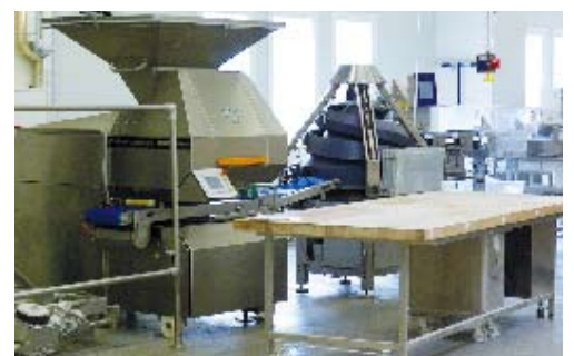
The bread line with V700 hydraulic divider and conical round moulder. The multiple-way system allows the production of tin products, directly proofed breads or breads proofed in baskets in different shapes.
