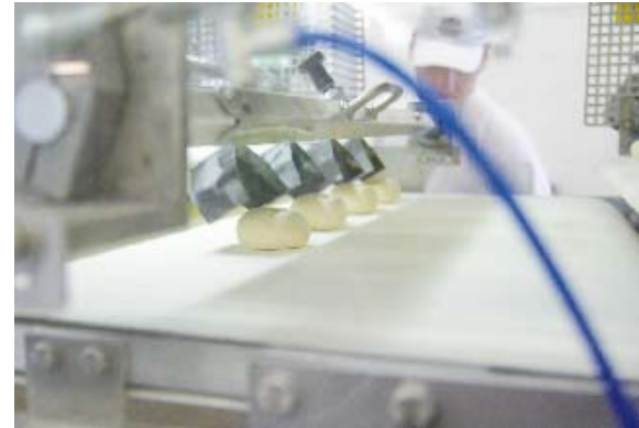
Production of Kaiserbrötchen (bread rolls with star incision): Before stamping the dough pieces are turned and aligned in one row.
