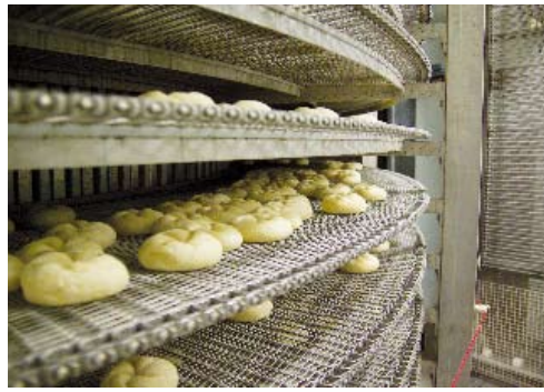
In the cooling spiral the bread rolls are cooled down to room temperature and afterward consigned in the shipment department.
