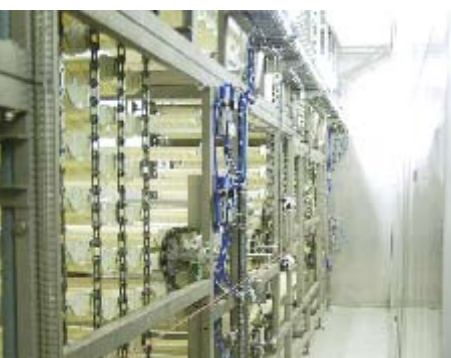
The final proofer for small products. Before the end of the proofing time there is the possibility to turn the dough pieces.
