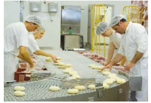
In the cooling spiral the bread rolls are cooled down to room temperature and afterward consigned in the shipment department.
