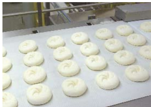
Completely proofed, the big volume dough pieces leave the proofer and are deposited onto the infeed belt of the oven loader by means of a crosswise retracting belt.
