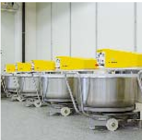
The dough preparation of the SPAR bakery in Ljubljana. Here, long bowl proofing and the use of pre-dough determine the production of the dough.
