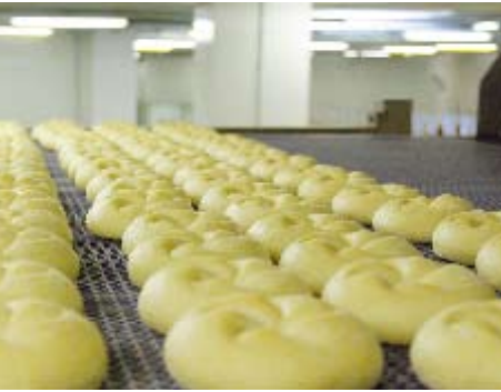
After baking the Kaiserbrötchen (bread rolls with star incision) have a uniform pale coloration all around and a product stability without marks of collapsing.
