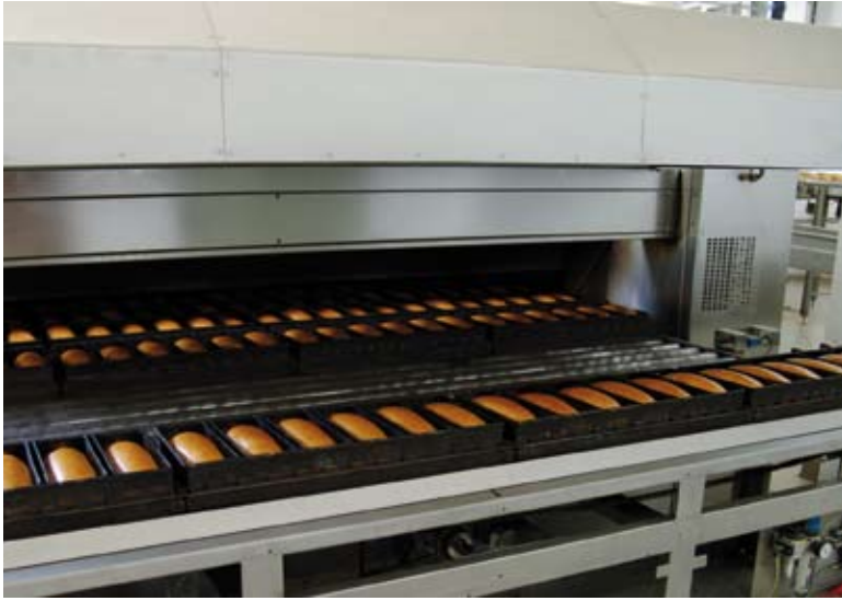
To allow for the production of both products on one line, WP installed a Duo-therm tunnel oven for products on trays and in tins.
